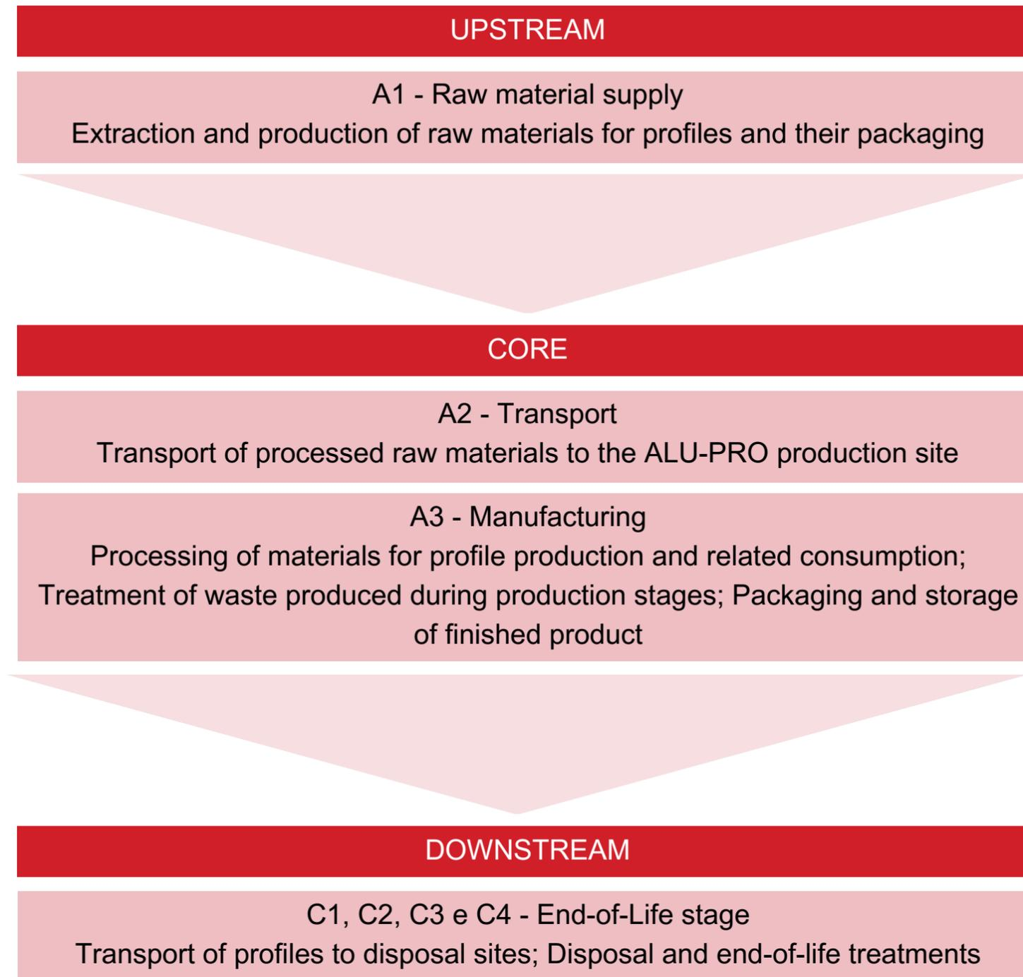
Figure 2 - System boundaries of the 4 analysed spacer profiles.
