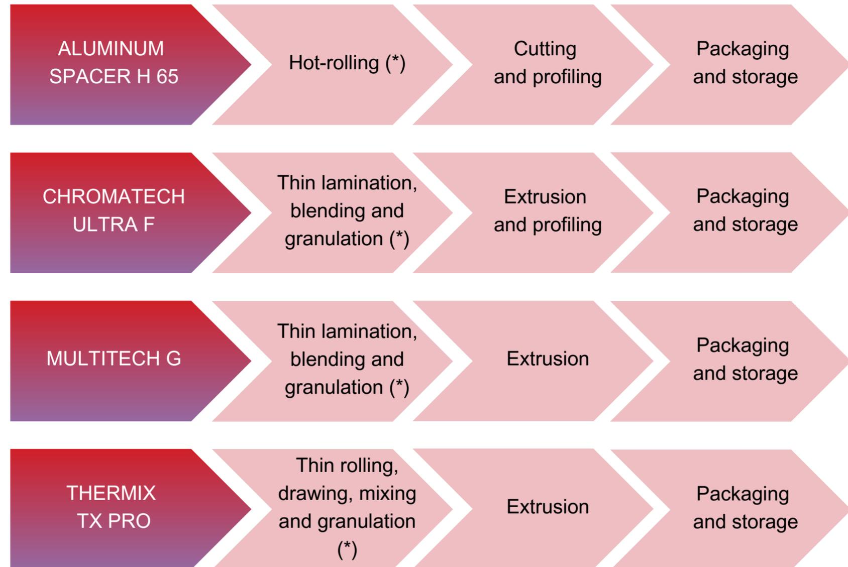
Figure 1 - Summary of the main production processes of the analysed profiles. Steps marked with (\*) are not carried out by ALU-PRO.
